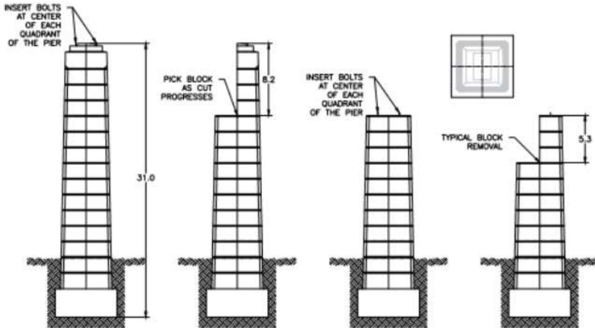
Figure 14 – Section 6 – Pier sawing
