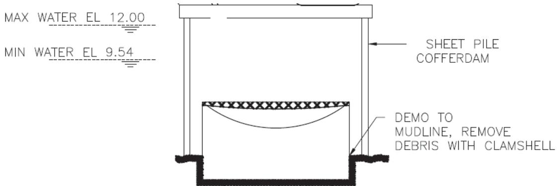
**Figure 17 – Cofferdam to be used for footing demolition**
