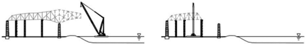
Figure 11 – Section 6 – Reverse erection of main span
