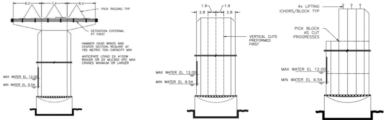
Figure 13 – Section 5 – Pier sawing
