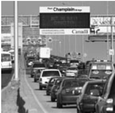
Typical rush hour on the Champlain bridge in Montréal. The variable message signs keep bridge users informed on traffic conditions ahead and potential alternative routes
