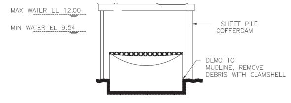
Figure 17 - Cofferdam to be used for footing demolition
