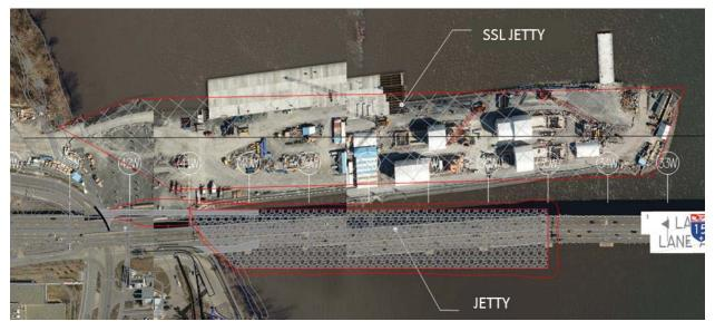
Figure 2 - Drawing - Proposed jetty on the Nuns' Island (IDS) side - photo: April 2016
