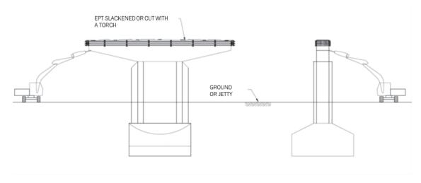
Figure 12 - Standard method - Foundations over land - Front and side views
