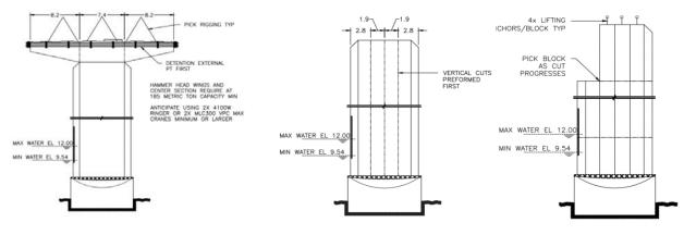
Figure 13 - Section 5 - Pier sawing
