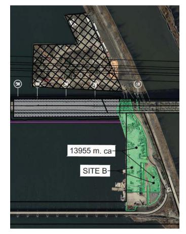
Figure 6 - Mobilization area and dismantlement and handling site "B" - Seaway dike
